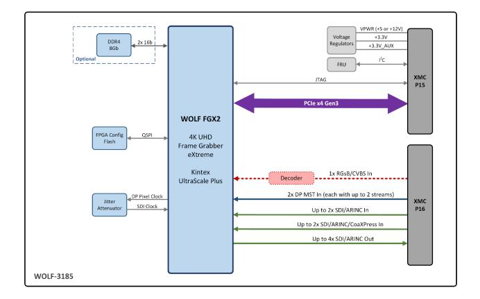
The number of simultaneous video I/O possible is constrained by both the number of physical connections available (as shown on the block diagram) and by the total bandwidth of the PCIe connection used to carry the active video data to the host system and back to the FGX2. For this XMC module there is a PCIe Gen3 x4 bandwidth of 31.5 Gbps for data that will be sent to/from the module.
