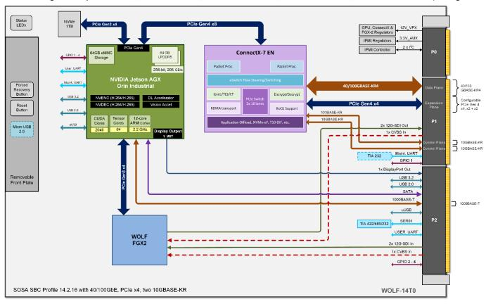
The following model provides two 10GBASE-KR, one 1000BASE-T and PCIe Gen4 x8 (configurable).
