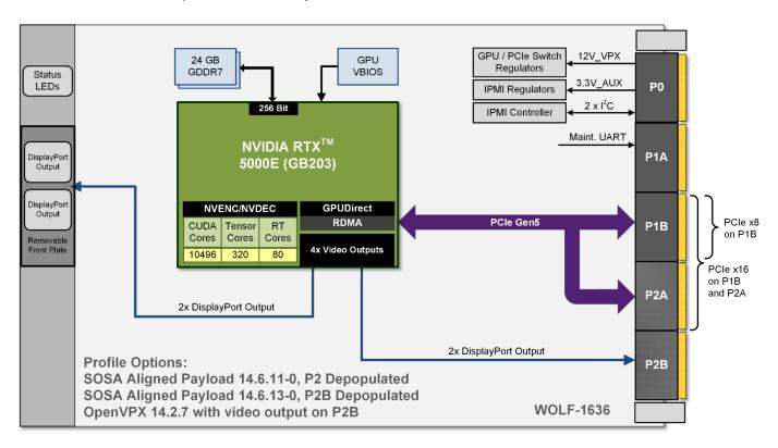
The OpenVPX profile supports DisplayPort video output, with two outputs supported on the rear connector, and two supported on the front panel under a small removeable panel. Note that the P2B pin assignment used for the DisplayPort video output for this product is not pin compatible with the previous generation WOLF-1538/1448/1348.
