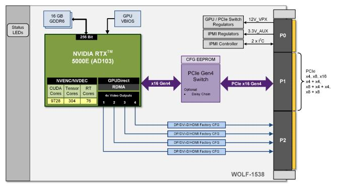
The OpenVPX model supports DisplayPort/HDMI/DVI video output.
