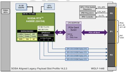
SOSA aligned model with support for Legacy Payload Slot Profile 14.2.3. The P2 connector is populated and can be used for video output.
