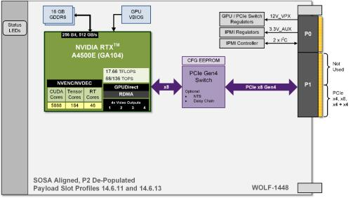
SOSA aligned model with support for Payload Slot Profiles 14.6.11-0 and 14.6.13-0. The P2 connector is de-populated and operates in headless mode.
