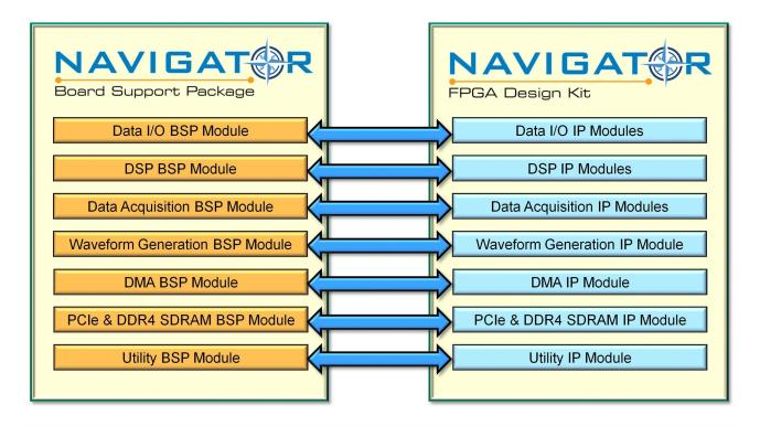
Because all Pentek boards are shipped with a full suite of built-in IP functions and numerous software examples, new applications can be developed by building on the provided software examples or built entirely new with the BSP's extensive libraries. All BSP libraries are provided as C-language source for full access and code transparency.
