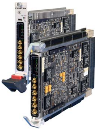
Model 53861 COTS (left) and rugged version
