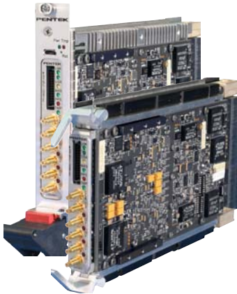
Model 53721 COTS (left) and rugged version
