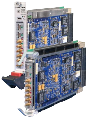
Model 53671 COTS (left) and rugged version
