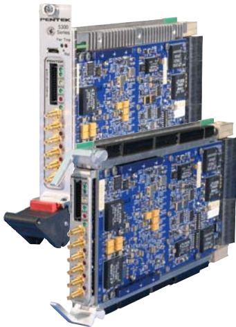
Model 53662 COTS (left) and rugged version
