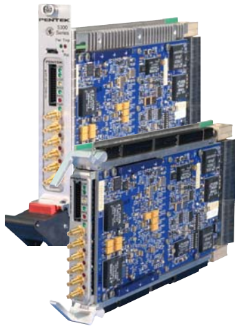
Model 53661 COTS (left) and rugged version
