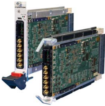
Model 52862 COTS (left) and rugged version
