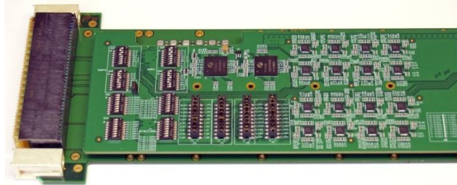
Picture 1: Switched lanes Mezzanine
