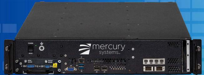
A part of the *EnterpriseSeries™*, Mercury's fanless RES Aero 2U Server employs Intel® Xeon® E5-2600 processors to silently accelerate compute intensive workloads for airborne applications such as surveillance, signal intelligence, sensor fusion, and audio/video processing.
