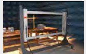
Radiated Susceptibility: Radiated H field 30Hz - 150kHz, 2MHz - 100MHz.
