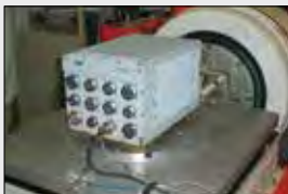
Vibration: X-Axis. 12grms @ 15Hz to 20kHz, 1 hour per axis.
