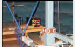
Radiation Emissions: Radiated E field 30MHz to 1GHz vertical polarization.
