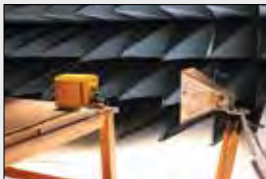
Radiated Emissions: Electric field, HORN, 1GHz up to 18GHz.
