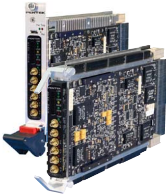
Model 52821 COTS (left) and rugged version
